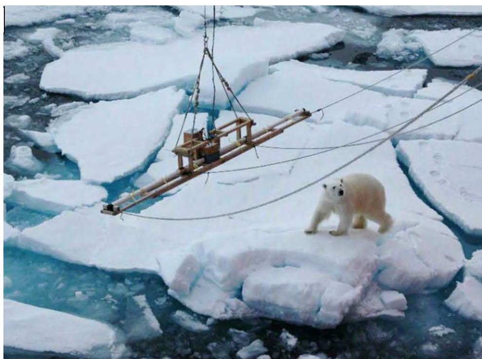
A polar bear with an electromagnetic induction ice thickness profiler photographed in the Canada Basin on August 18, 2008
