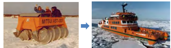
Fig. 6 Archimedes' screw vehicle was developed to Sightseeing Icebreaker Garinko.
