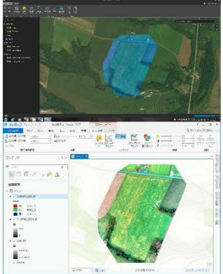
Fig. 7 Orthomosaics from drone-captured imagery
