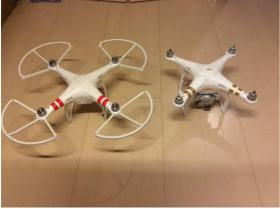
Fig. 1 DJI Phantom quadcopter (Version2: Left and Version3: Right)
